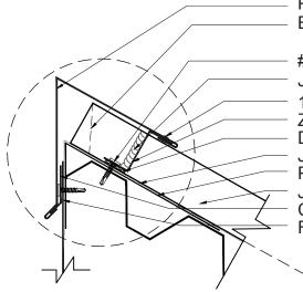
Peak Flashing Box End of Panel (See Zee Closure Options Detail)
