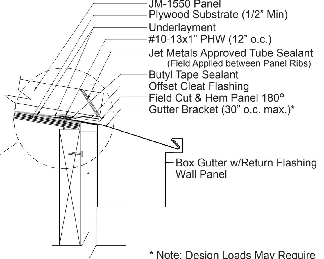
Box Gutter w/Return Flashing
