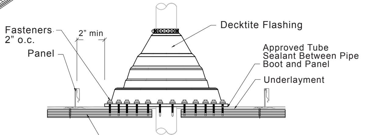
Existing Plywood Deck, Cut Hole in Deck at Least 2" Greater than Pipe Boot Flange
